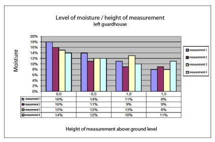
Fig. 7. Level of moisture / height of measurement – left guardhouse. Bar graph as per information in Zaród [13]
