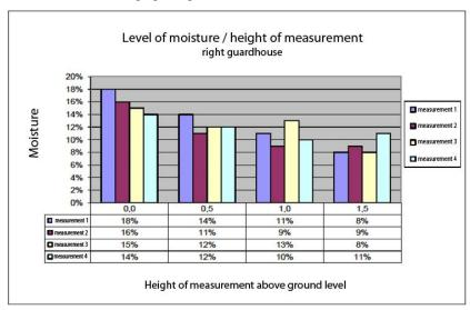
Fig. 8. Level of moisture / height of measurement – right guardhouse. Bar graph as per information in Zaród [13]
