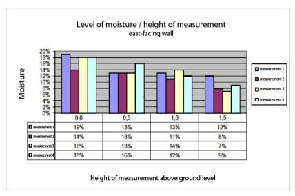
Fig. 3. Level of moisture / height of measurement – east- facing wall. Bar graph as per information in Zaród [13]
