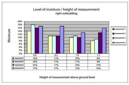
Fig. 6. Level of moisture / height of measurement – right outbuilding. Bar graph as per information in Zaród [13]
