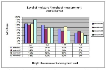
Fig. 4. Level of moisture / height of measurement – west-facing wall. Bar graph as per information in Zaród [13]
