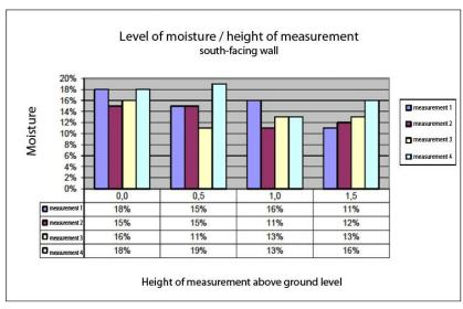
Fig. 2. Level of moisture / height of measurement – south- facing wall. Bar graph as per information in Zaród [13]
