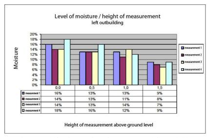
Fig. 5. Level of moisture/ height of measurement – left outbuilding. Bar graph as per information in Zaród [13]
